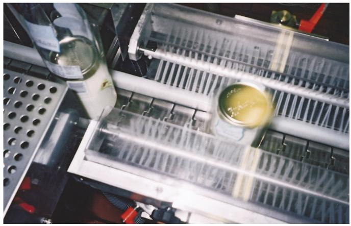
Bottles leaving the labeler move through a flail device consisting of rotating brushes on both sides of the conveyor that push the labels down to be flush against the conveyor surface.
