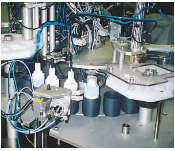
This is the last monobloc in the system. The stems, which are the only component supplied in a roll, are inserted at this station, as well as an internal component and the overcap.
