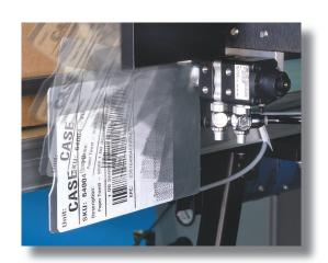
We've even engineered an exclusive system that prints, encodes, verifies and applies smart labels in a single operation. And when the encoded RFID tag is not verifiable, a unique swing plate automatically intercepts the smart label *before* it's applied.
