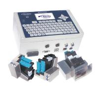
Ink-jet printer Designed for primary package coding, the HPbased Jetpack1000 ink-jet printer features multiple time and date stamps, and lot number and incremental numbering capabilities. The printer also prints bar codes, graphics and logos at up to 12 lines/printhead. Compact Flash and Ethernet interfaces are available. Prism, Inc.,
