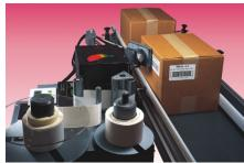
The AD-2800 high speed, high-volume. roll-on applicator features precise placement of pressure-sensitive labels. Ideal for applying labels to flat and cylindrical products. The CPA-350 automates printing and application of pressure-sensitive labels. Userselectable application settings, and choice of print engines. Backed with QuickLabel's manufacturer-direct enduser service and support.
