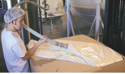
After the tote and cassette are in place on a pallet and the product is blended and pumped from a nearby tank, a hose is connected to the filling valve in the top of the collapsed liner, far left. Then, the operator starts the pump for a 330-gal fill. As the liner fills from the bottom up, near left, the operator has time to go to work on other tasks.
