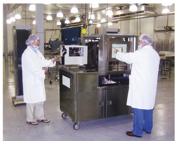
Beaver Street Fisheries personnel use a portable, cart-mounted RFID-tag printing/encoding station on a slap-and-ship basis to generate smart labels for cases of frozen seafood that it ships each month to a Wal-Mart distribution center.
