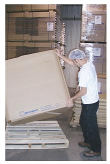
An operator sets up the 330-gal container's outer shell on a pallet. The totes hold product mixed in two stages.
