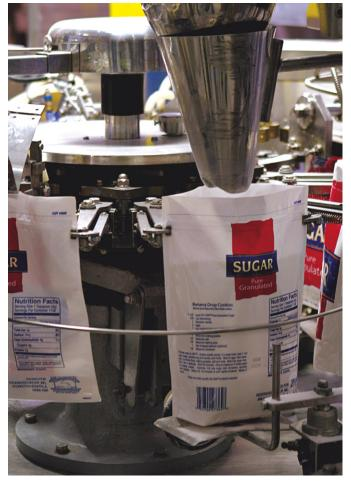
One of two semi-automatic fillers at Flex Pack, above left, fills 16-oz bags of powdered sugar. For 10-lb bags of white sugar, the company uses its new automatic filling machine, above right, that requires operator intervention only to feed bagstock. The machine uses gripper arms to hold the bags open, left, while sugar is dispensed.
