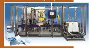
The output of both wrapping legs feeds into two collators, where a robot arm with a customized gripper toploads the vials into the cartons. After a leaflet is inserted, the carton is closed and case-packed. Cases are erected, bottom-glued with hot-melt adhesive and top-loaded in two layers. After being bar-coded for traceability, a corner label is applied and the case is automatically palletized. A Cognex (www.cognex.com) vision system verifies lot codes and expiration dates.
