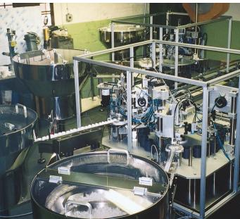
Pucks are used to transport the caps through the entire assembly process. Each indexing monobloc consists of five to seven assembly stations designed to add parts to the traveling puck. The monobloc shown in these photos is the second in the system.
