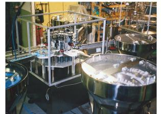
The system to produce the pumping cap, right, incorporates interconnecting and synchronized indexing, rotary, cap-assembly monoblocs with 10 vibratory bowls and a web feeder to automatically unscramble and/or feed parts to the monoblocs. The machine, left, which includes four bowl feeders, is the first monobloc in the system.
