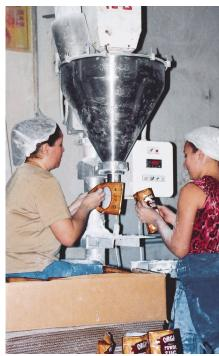
A new servo-driven pouchmaking machine, left, can create bottom-filled or three-side-sealed pouches at up to 4,800 bags/hr. The semi-automated auger filler, above, is used to fill short runs, nonwhite, granular sugar and other dry products in pouch sizes from 14 oz to 25 lb.
